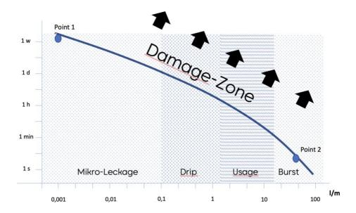
The diagram above shows the relationship between flow speed of water (in liter/minute) and the time this water flows out. The thick curve marks the area where damage will happen (about 10 liter of water, one full bucket). The required reaction time to a detected leak depends on the flow speed of the water. For micro leakages - point 1- its ok to act after few days or even weeks while a fatal burst of a pipe requires a reaction within seconds – point 2.
